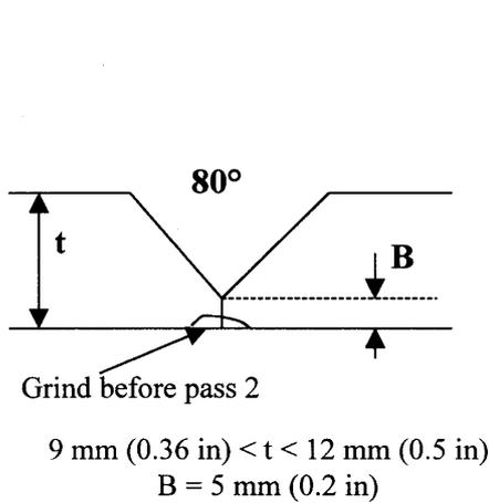
E. Suitable for SAW. Grinding after first pass facilitates full penetration.
