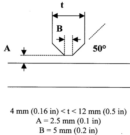
F. Full penetration Fillet. Suitable for SMAW. Tack weld with SMAW or GMAW.
