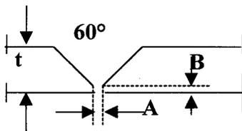
G. Single V Joint. Pipe welding. Suitable with SMAW.
