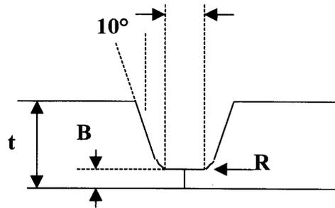
H. Single U Joint. Pipe Welding. Suitable with GTAW.
